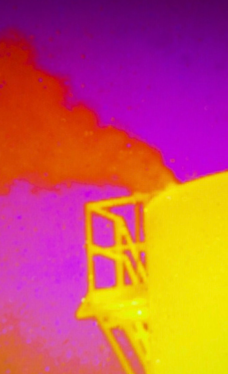
Infrared thermal image of methane gas leak, otherwise undetected, at fracked gas facility in New Mexico. Photo by Shaun Stanley
